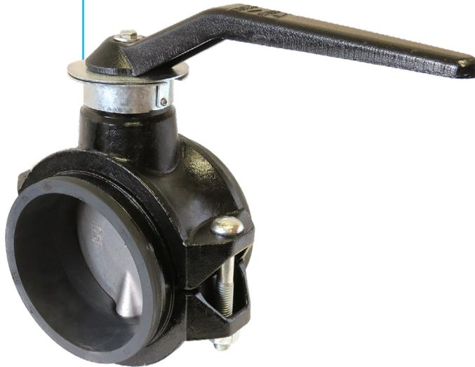
The Fig. 70G Butterfly Valve is designed for use with Gruvlok couplings, an ASC Engineered Solution, for fast and easy installation on grooved pipe. The valve body is fully rubber lined in EPDM or Nitrile material. A 316 Stainless Steel Disc is standard. The valve is supplied with a two position lockable handle.
